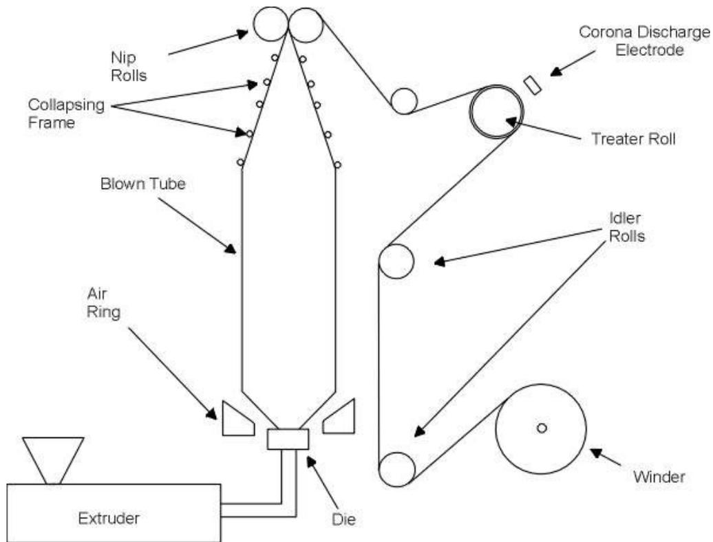
**Figure 3: Line Schematic – Top of the Tower Treatment**
