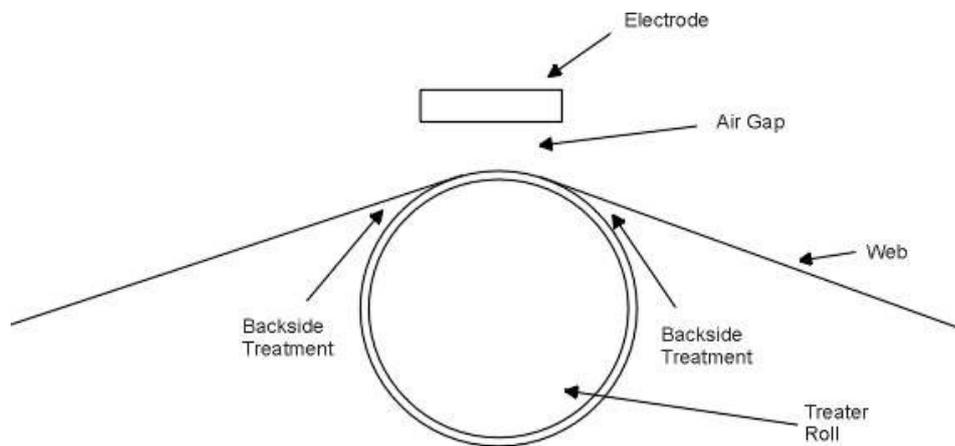
**Figure 5: Insufficient Wrap leads to Backside Treatment**
