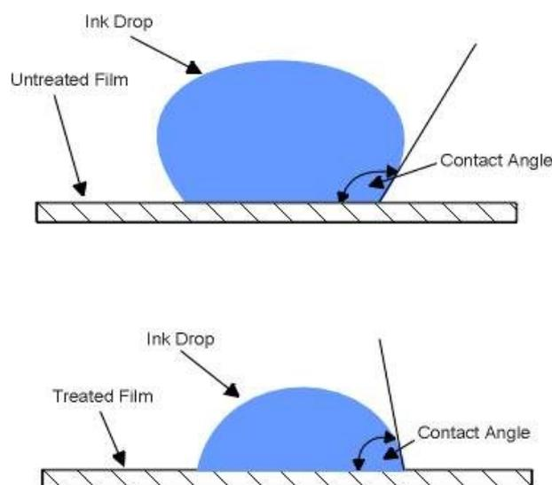
**Figure 1: Schematic Representation of Surface Tension**
