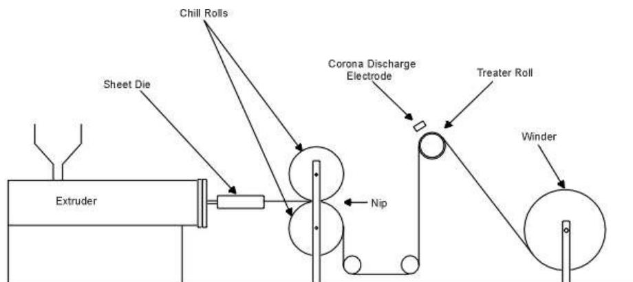
**Figure 4: Sheet Extrusion Line**
